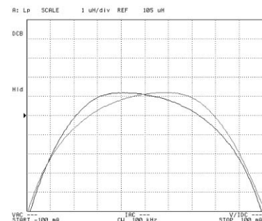
Inductor DC dependency characteristics (100 μH inductor at 100 kHz) UP and DOWN DC current bias sweep from -100 mA to +100 mA. Hysteresis is observed.
